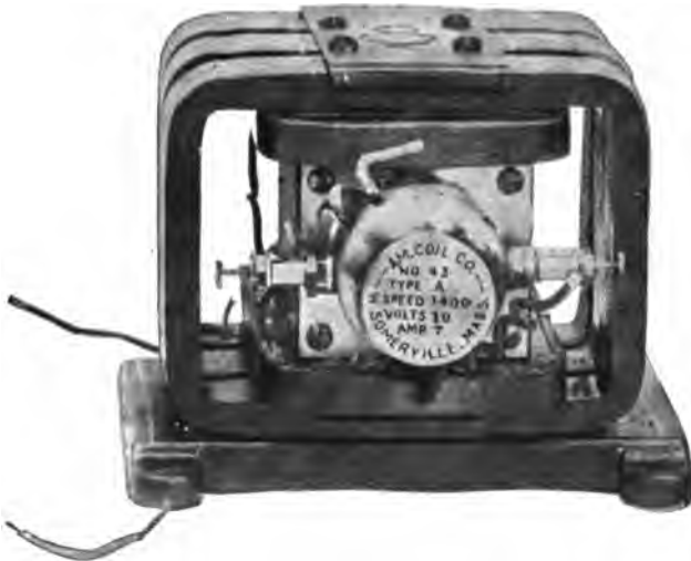
FIG. 340.—The American "Little Giant" Ignition Magneto. This generator consists of six magnets placed end to end as shown. An armature of the ordinary dynamo pattern, rotates within the pole pieces, generating a powerful current at any speed between 800 and 1,500 revolutions per minute, and developing between 10 and 15 volts and from 6 to 8 amperes. By a combination of permanent magnets and field windings, the field is constantly maintained, while the spark produced is the most powerful that could be generated by any machine of its size and weight.
